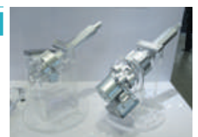
Force Feedback Actuator for Steer-by-Wire (left) Worm reduction gear type (right) Coaxial reduction gear type
